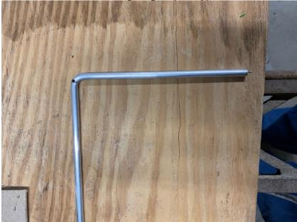
Step 4: unscrew the set screw enough to slip one on each end of the rod, pointing the tail of the lug away from the rod. Tighten both set screws enough to keep them on the rod, but not firmly at this point. Have both tails of the lugs, flat on your bench.
