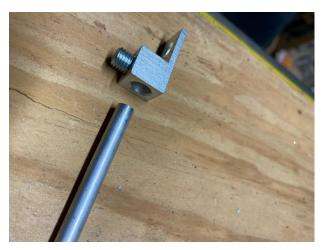
Step 5: Use the now assembled perch to mark your rack if necessary, and drill 1/4 inch holes to attach. If you have Gemini racks, use the holes already available. Attach the perch with the flat side of the lugs against the rack. Loosen the set screws if necessary, so that the lugs seat firmly to the rack, then tighten bolts and set screws firmly.
