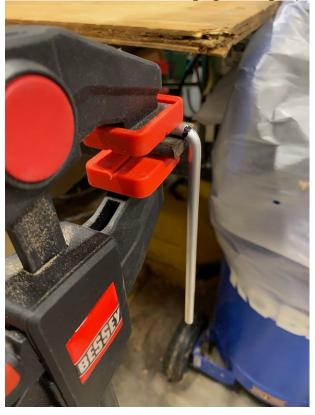
Step 3: With your palm placed near the marked spot of rod, bend the rod down to form a 90-degree angle. Repeat with the other end of the rod, paying attention that both bends go in
